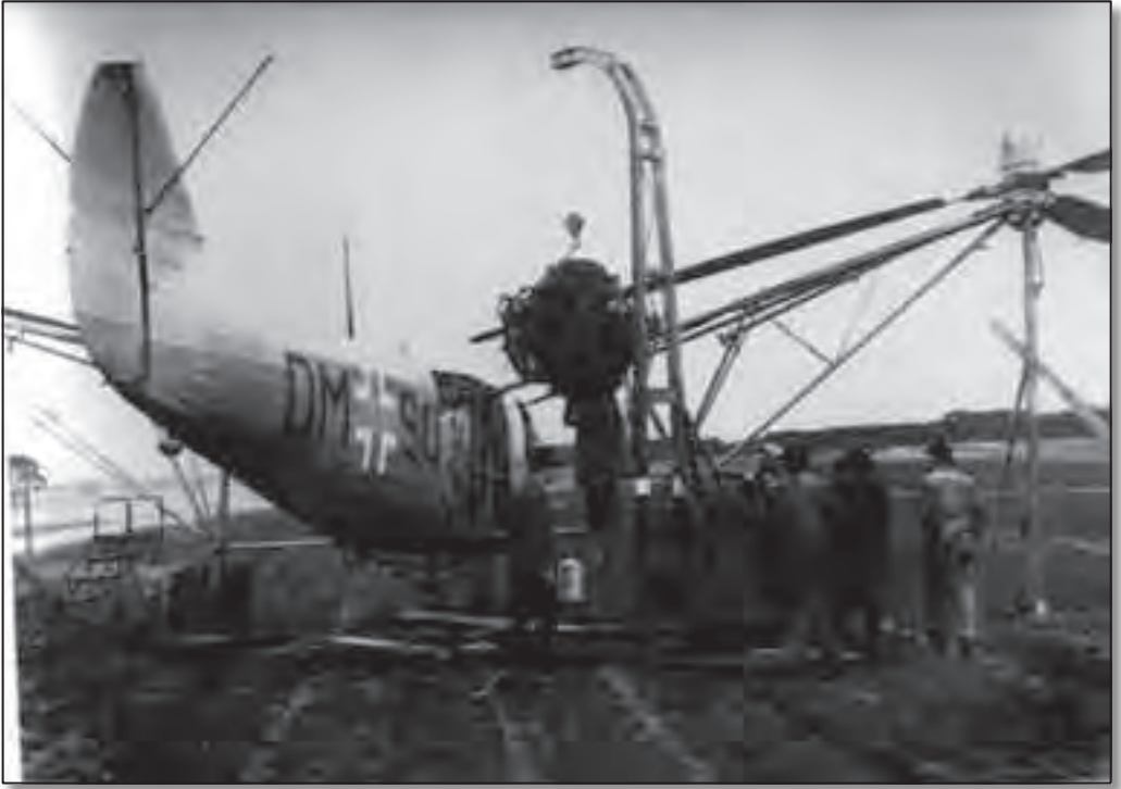
Fa 223 Drache V11 DM+SO during an engine exchange in the field.
