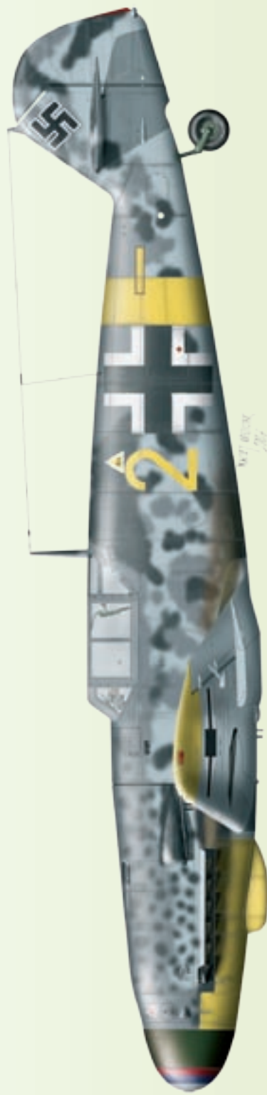
Messerschmitt Bf 109G-4, "yellow 2", of 13. (slow.)/JG 52 in April 1944, when the Squadron operated from Anapa airfield, Kuban. It sports the standard Luftwaffe camouflage, i.e. the upper surfaces RLM 74 (Graugrün), and RLM 75 (Grauviolett) paint, the side and the lower surfaces in RLM 76 (Lichtblau), on which the irregular mottle of RLM 74, 75, and RLM 02 (Gru) are visible. The lower cowling, the stripe on the fuselage and the wing tips were painted yellow (RLM 04- Gelb), characteristic of aircraft operated on the Eastern Front. The only sign that the aircraft is flown by the Slovaks is the spinner's front part, painted with the Slovak national colours (white, blue and red), while the rest of the spinner remained in the original RLM 70 (Schwarzgrün).
