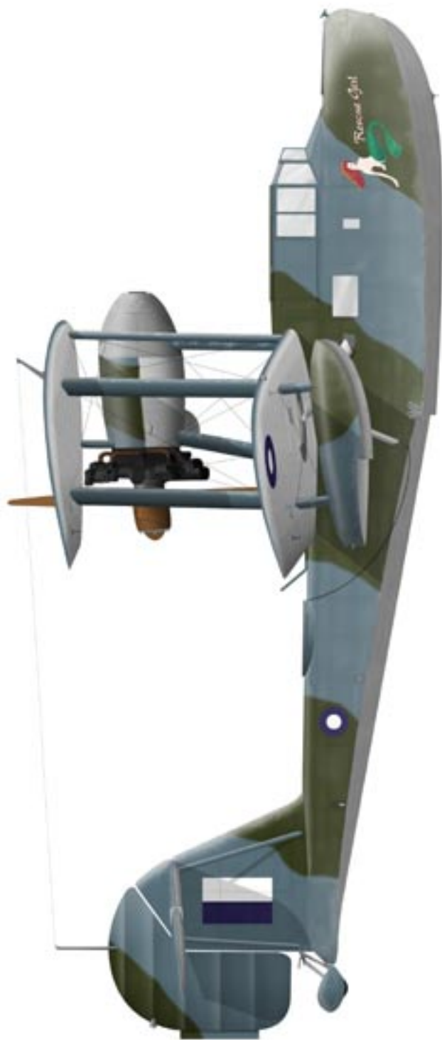
RAAF ASR Walrus Mk.I „Rescue Girl” (unknown serial) serving with 71 Wing in the Admiralty Islands, Sept 1944. Colours of the mermaid are unconfirmed. Note the primer painted front half of the engine nacelle.
