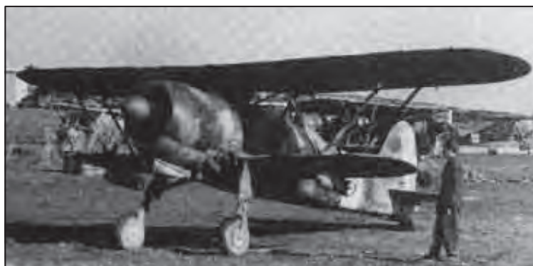
Fiat CR.42 AS with the wheel fairings removed and with the 100kg bombs under the wings.
