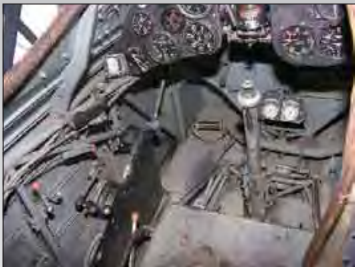
Left: Another view of the cockpit of the Swedish Falco. The control column and rudder pedals are visible. Note also the left side panel with engine control levers.
